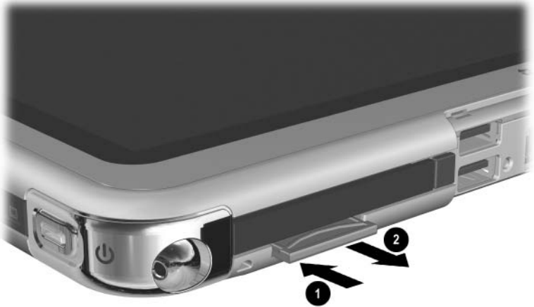
Releasing the SD Card (space saver shown)
